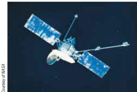
Figure 34.9 Mariner 10 used its solar panels to "sail on sunlight."
